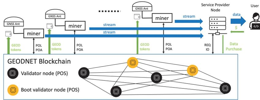
FIGURE 5 GEODNET architecture: Miners, validators, and service providers
