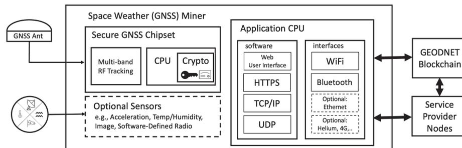
FIGURE 2 Space weather (GNSS) miner architecture
