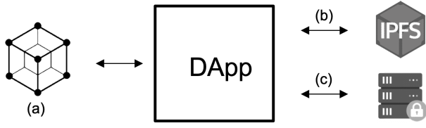
Figure 2: Typical structure of nodes/services required to run a DApp, such as a marketplace: (a) a consensus node, e.g., an Ethereum node; (b) an IPFS node, for NFTs implementing pattern (2); (c) access to privately-owned internet servers, for NFTs implementing pattern (3).
