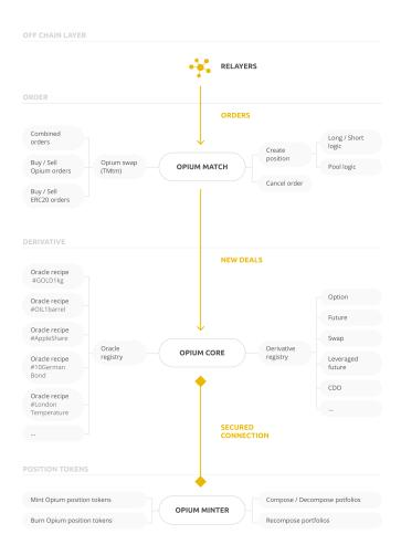
Figure 3: Technical schematic of Opium Protocol
