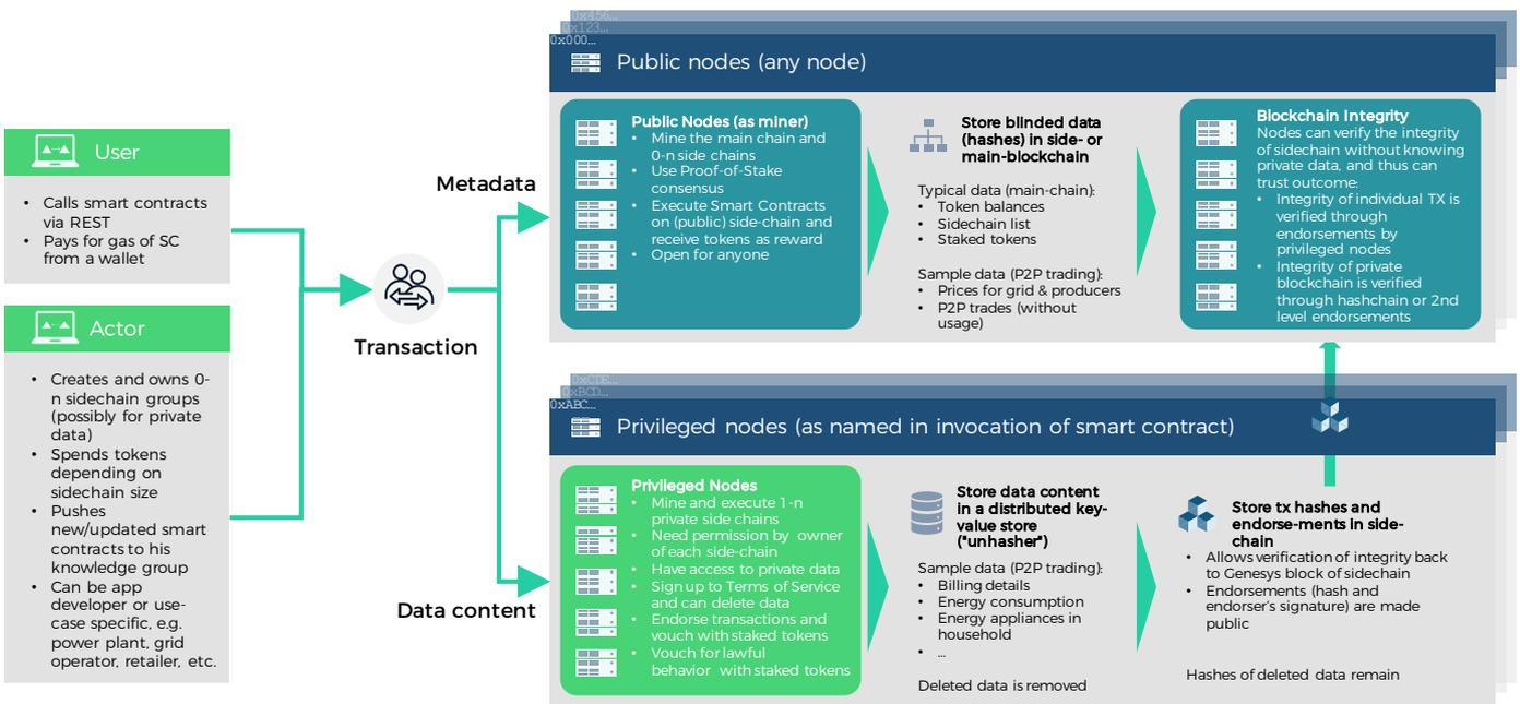
Figure 5: Lition blockchain data separation and deletion concept
