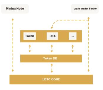
The construction of DEX architecture on LBTC can be divided into four levels.
