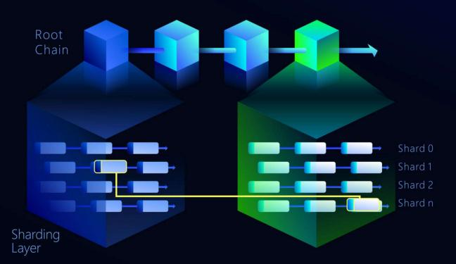
Fig. 8 Illustration of cross-shard transactions, where the output of the transaction can be spent as long as the cross-shard transaction is confirmed by the root chain.
