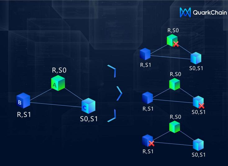
Fig. 7(B) illustration of high availability of a cluster with 2 shards run on the QuarkChain Network, where the cluster could still fully validate the network even any single node is crashed (right). For example, suppose there are 2 shards in the system, A validates shards 1-2, B validates shards 2 and root chain, and C validates shards 1 and root blockchain, and A,B,C are honest to each other, then A,B,C could form a cluster that is able to fully validate any blocks.
