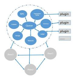
The underlying development framework of blockchain using plug-in technology, which keeps the main function of blockchain and adds plugins as extended functions.
