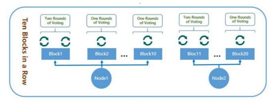
When the consensus node is used as a Proposer, it continuously proposes and packs multiple blocks. The first block is confirmed by two rounds of voting, and the subsequent blocks are confirmed by one round of voting.
